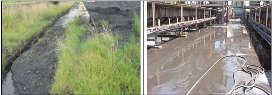
Figure 6-12: Examples of poor water conveyance practices
