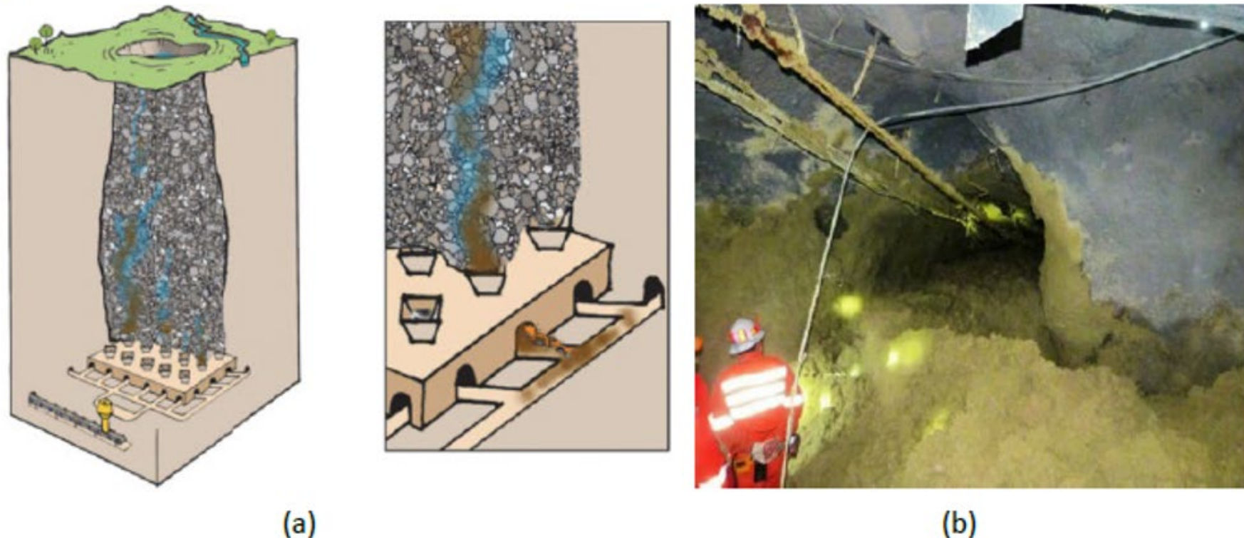
Figure 1 (a) Schematic representation of water inflow into the broken ore columns and the occurrence of a mudrush (Flores-Gonzalez 2019); (b) Occurrence of a mud rush at a drawpoint in the extraction level during mine operation in El Teniente mine (Codelco 2016)
