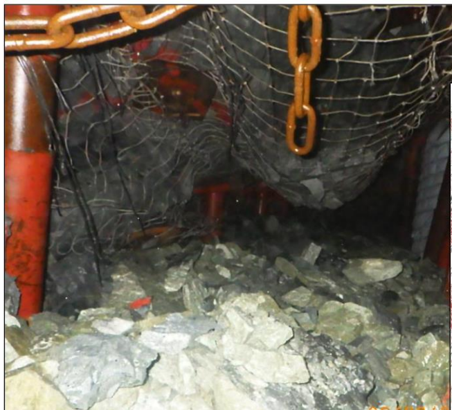
Examples of post-seismic events at Masakhane where the nets have caught falling rock.
