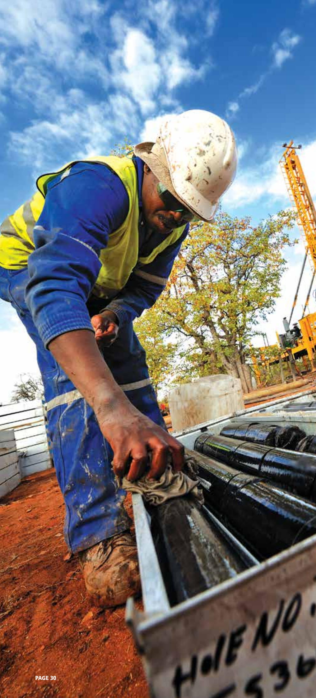
Cleaning core samples at Coal of Africa's Makhado project in Limpopo
