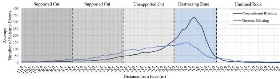
Fig. 7. Average number of seismic events per development cycle for both conventional and face distress blasting techniques.
